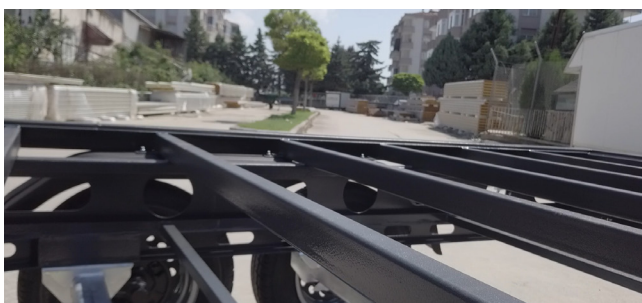
Chassis are built by using ST52 & ST37 laser cut steel
